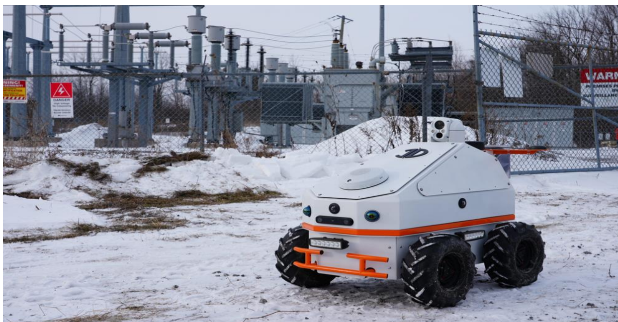
Above, InDro's dual-purpose Sentinel inspection robot, which can map environments and detect anomalies, illustrates this crossover.
